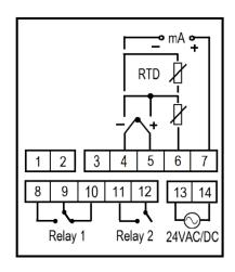
PT100: both R1 resistors must be equal, but also if needed R1=R2
